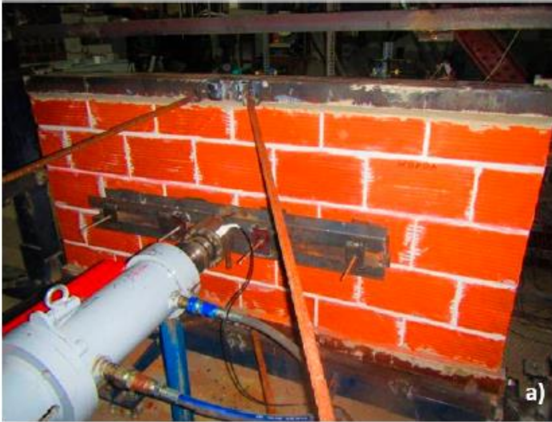
Figure 4. Used loading arrangement (steel strong reaction frame) for the out-of-plane flexural performance of masonry wallets with or without thermo-insulating attachments. (a) View of the facade without thermo-insulation where the actuator is attached. (b) View of the facade where the thermo-insulation is attached.
